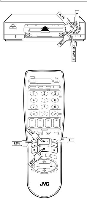
The easiest, most basic operation possible with your video recorder is tape playback. Already-recorded signals on a video tape are read by your video recorder and displayed on your TV just like a TV programme.
