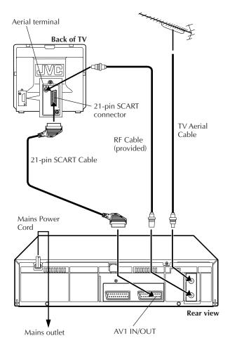
Make AV connection if your TV has a 21-pin AV input connector (SCART) in order to reduce the possibility of interference.
