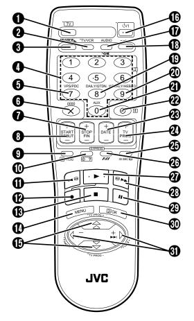
Buttons with a small dot on the left side of the name can also be used to operate your JVC TV while holding down the **TV** button.  $\square P$  "Operating JVC TVs" below.
